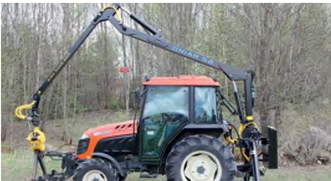
3-point mounting standard on most models. May require extra bracing kit. Can be used with PTO pump & tank.
