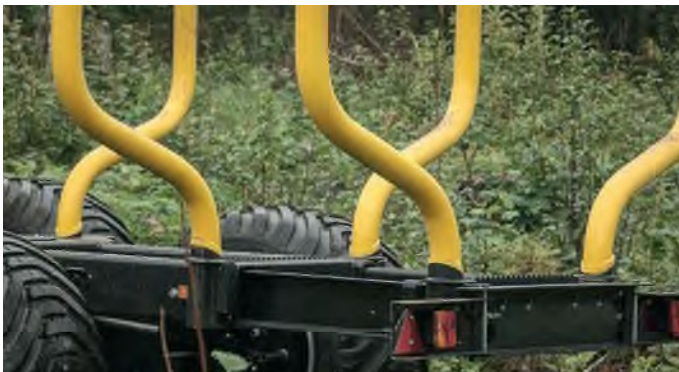
Optional rear frame extension for 10T, 12T and 14T trailers.
