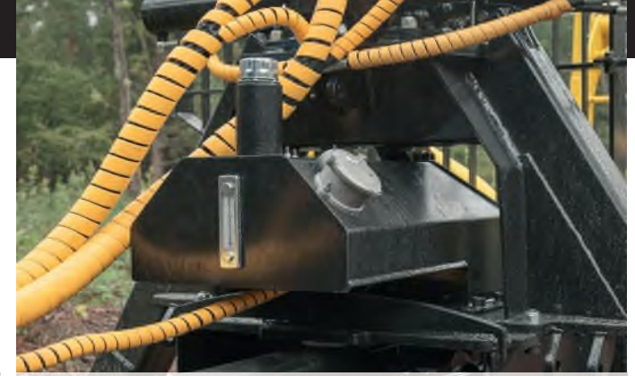
Optional independent hydraulic system driven by tractor PTO.
