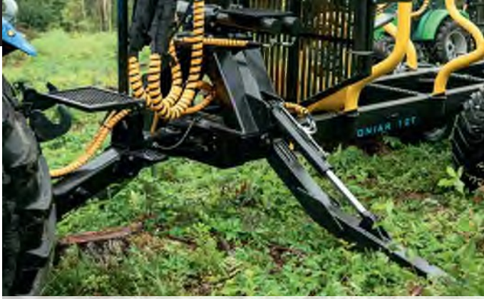
Wing type hydraulic support legs.
