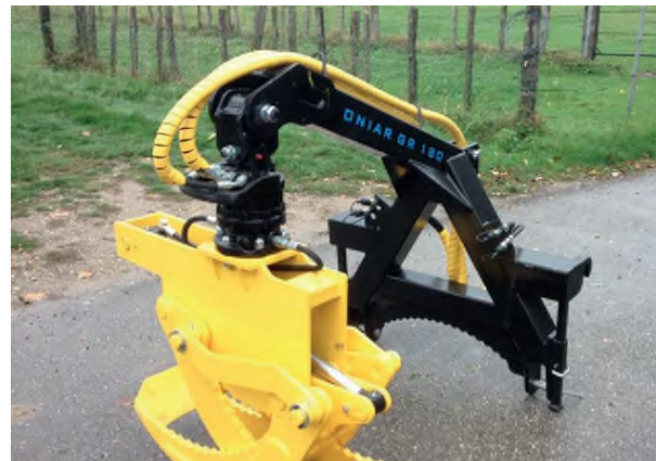
GR180 with 55 KNm rotator
