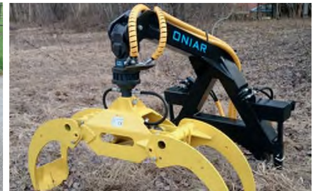
3-point linkage frame with 40 kNm rotator and G23 grab.
