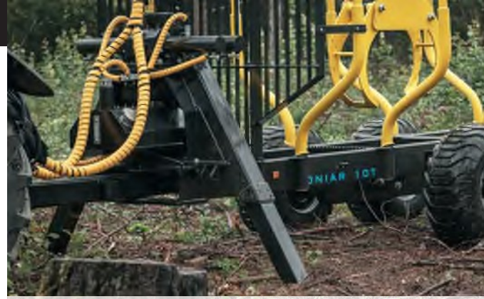
'A' type hydraulic support legs.
